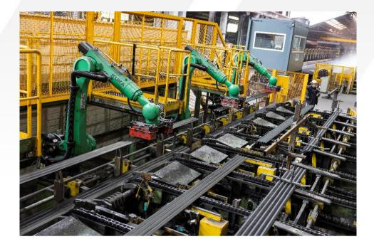
For this project, AIC installed an automation PLC and an integrated safety PLC on a Rockwell platform, with supervision plus Ignition recipe book. AIC also participated in the design of the electrical cabinet layout. All the drives are ABB, interfaced to the plc with Ethernet IP network, all the nodes are aimed at optimizing the plant installation, furthermore, local boxes were used to control the machines for man-machine interface with Ethernet IP nodes.
