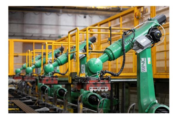
A special feature of the system is that it is able to shift from one profile to another: the set-up of the machine is very simple and fast to change, in 7 minutes a single operator is able to reequip the robot for a new profile. The system is very flexible, and depending on requirements it is possible to stack from above and below the profiles or alternatively stack it in a mixed way, this flexibility is useful to reduce stacking cycle times and to form tidier packs.
