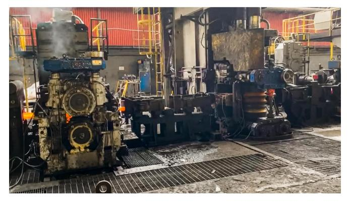
\* The initial phase encompassed the other 8 stands already existing on the site (3-6, 9-12), focusing on drive systems and motors by integrating renewed Siemens SINAMICS S120 modules of 800kW each. This phase also included equipping the stands with the existing PLC.
