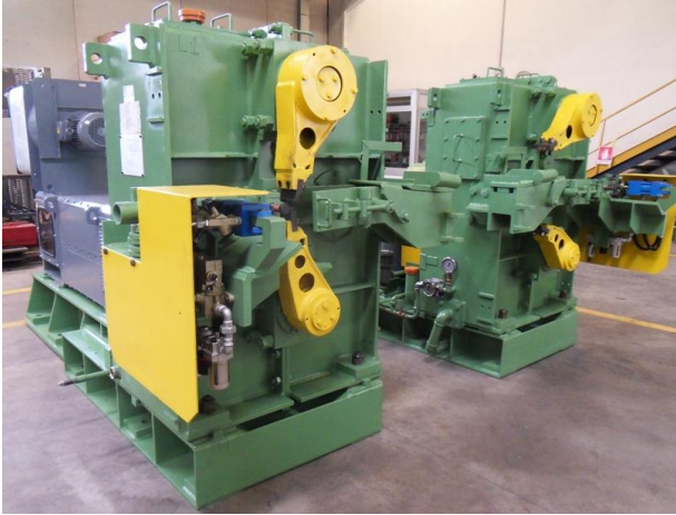
Fig. 17 – Shears after mechanical upgrade
