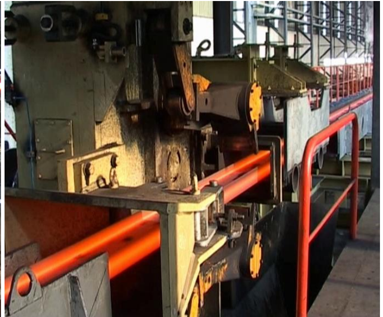
Fig. 19 – Example of Start/Stop shear for Bar Medium Section Mill
