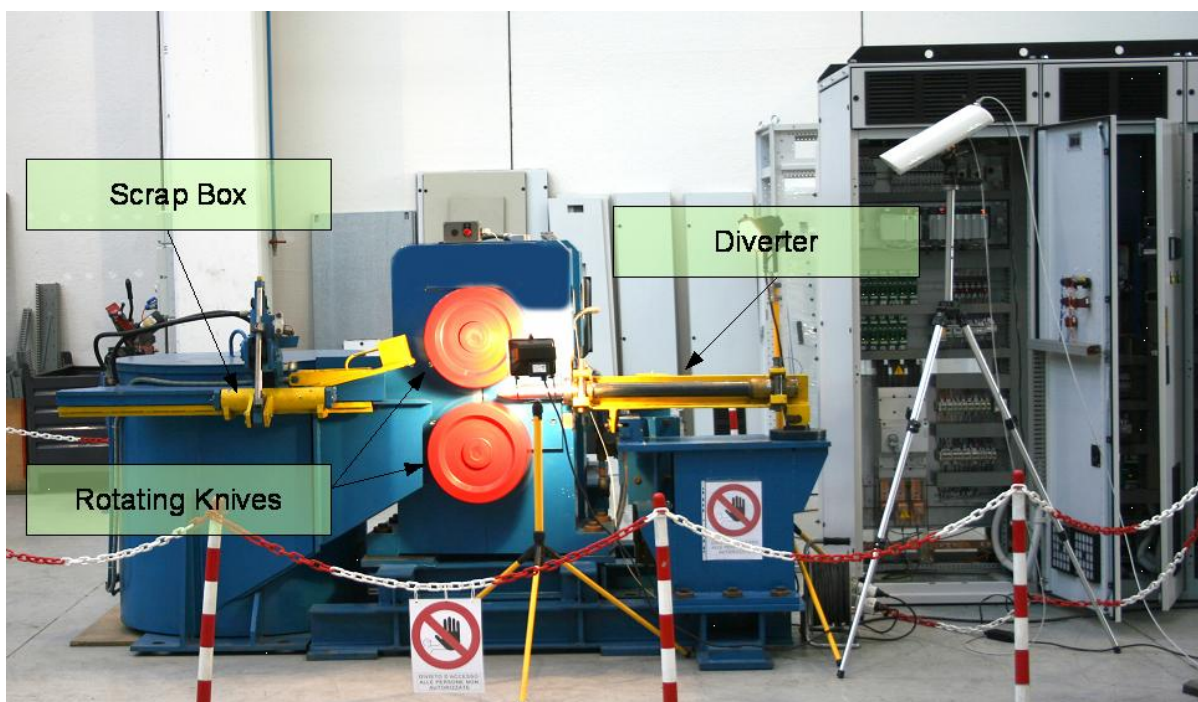
Fig. 4 – Example of rotating shear during the test phase in AIC workshop
