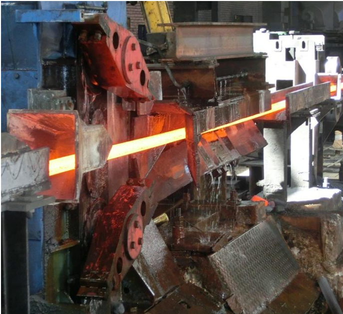
Fig. 19 – Example of Start/Stop shear for Bar Rolling Mill
