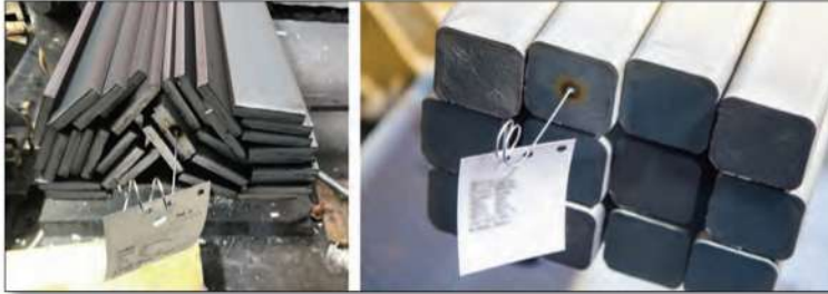
Fig 10 Tags metallic supports on bundles
