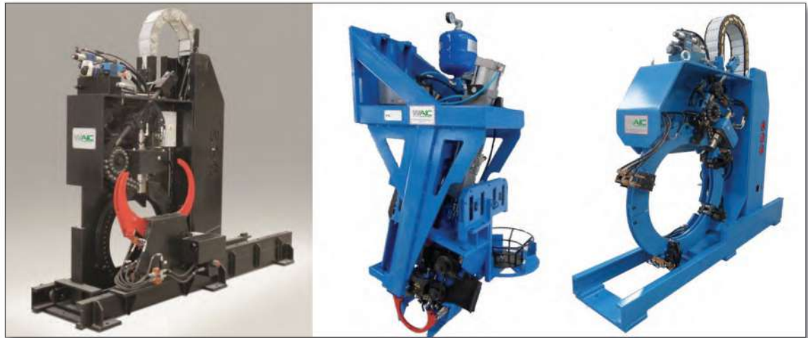
Ⓐ Fig 14 Tying machines for bundles, sub bundles and packs
