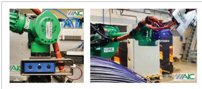
Fig 5 3D vision system during acquisition
