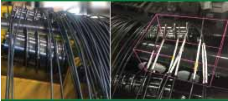
Fig 4 Photo of separated rings and the vision system interpretation of the same
